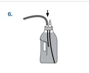
Attach the suction hoses to the adaptors on the cap of the Delivery Bottle. There are two hoses and two lengths of the tubes. First attach the hose with the half length tube to the bottle and suction through 1000 mL, then attach the suction to the second (longer) tube and suction through a 1000 mL. You may also use the second 1000 mL for treating the spittoon.
